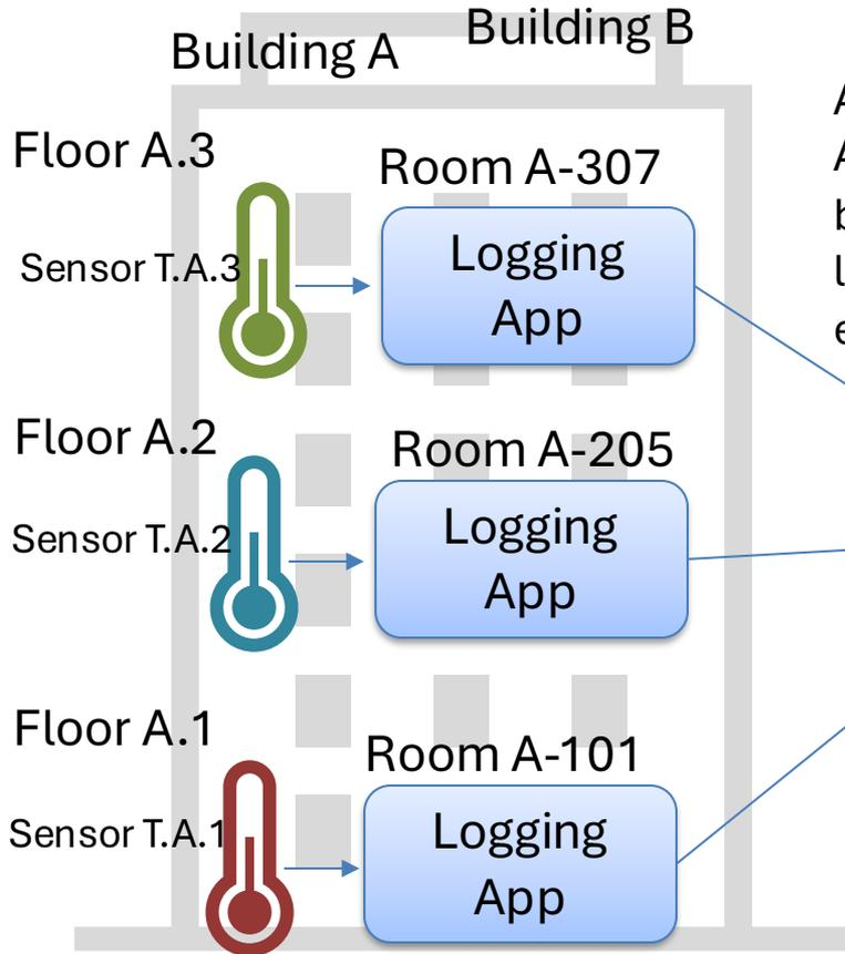
Assume that you can have multiple Data Logging Applications that are in different places inside multiple buildings (e.g., office buildings, factory, etc.) which are logging Temperature Data (or Data from other Sensors, CO2, etc.) and store the Data inside a common Database.
